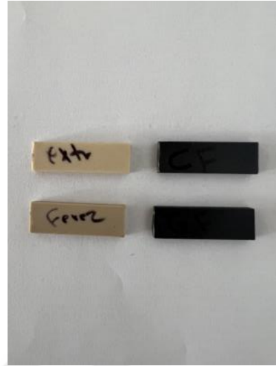
Figure 3.8 PEEK samples for hardness test
