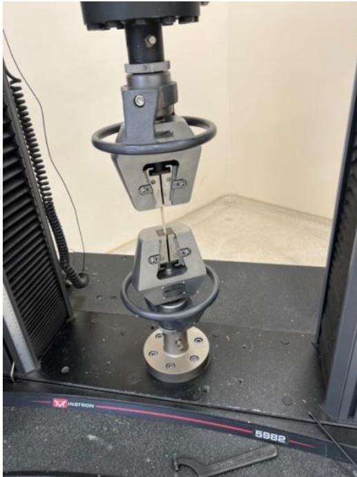
Figure 3.13 PEEK sample on tensile test
