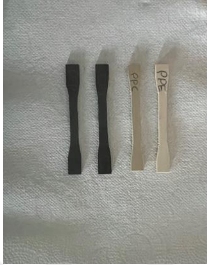
Figure 3.7 PEEK samples for tensile test
