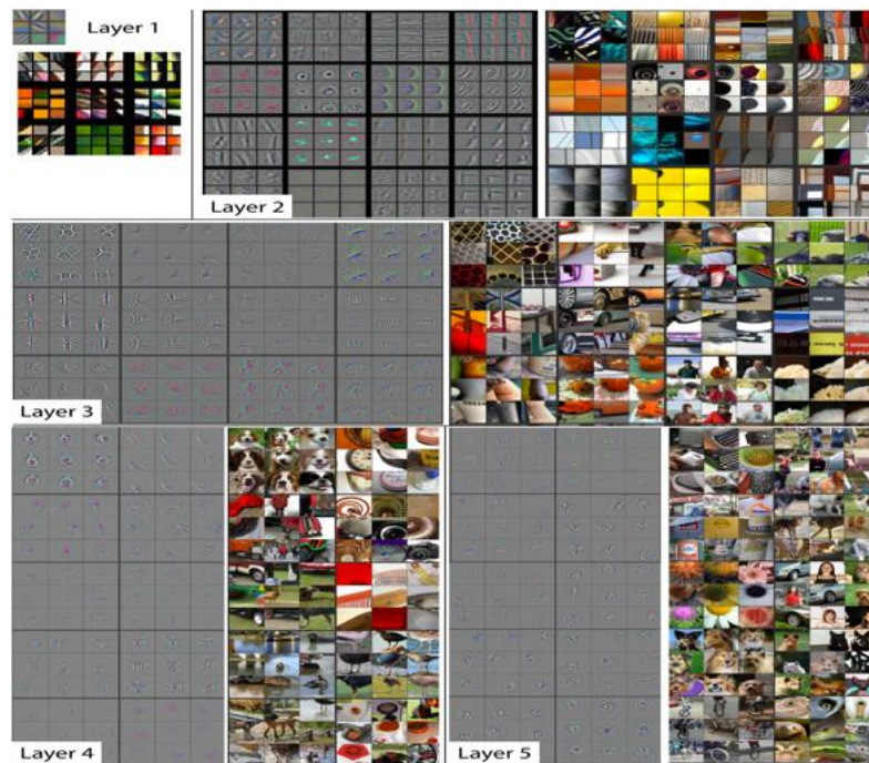
Figure 3.3: Visualization of the layer-based features by deconvolution and unpooling [177].
