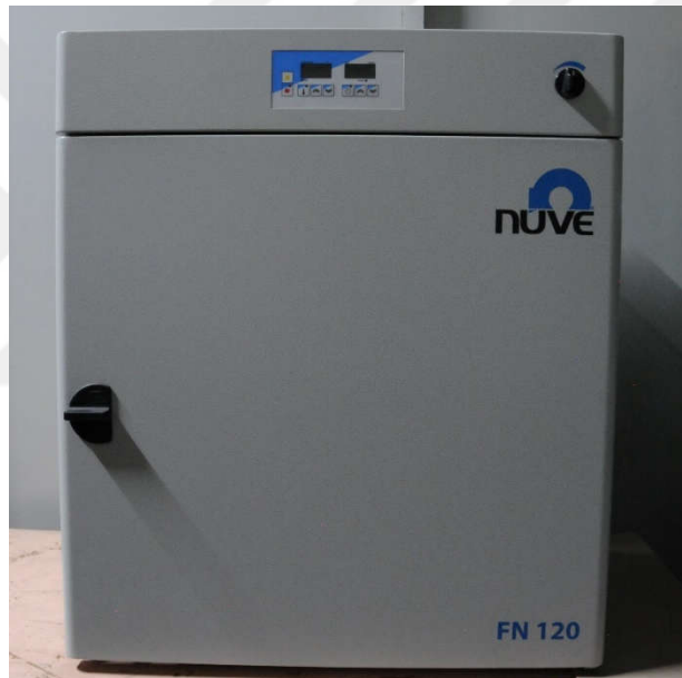
Figure 11. Oven used for measurement of wheat and fertilizer moisture content
