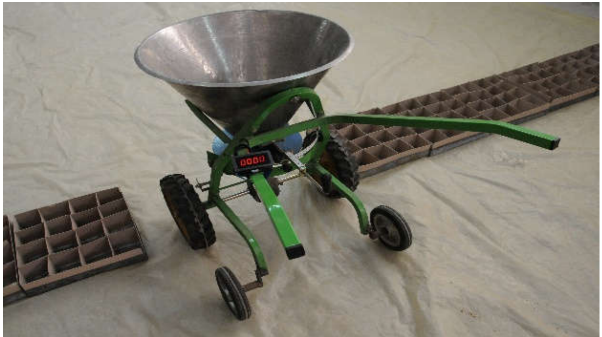
Figure 10. Proximity speed sensor for monitoring the spreader's forward speed
