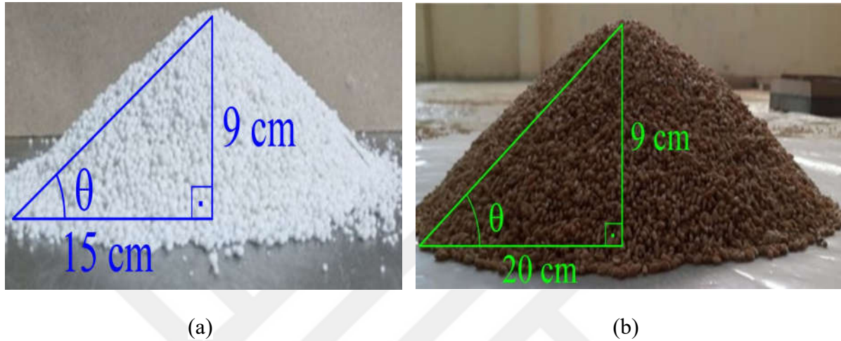
Figure 13. Repose angle of experiment materials (a) Fertilizer; (b) Wheat
