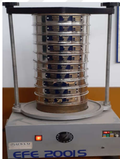
Figure 14. Vibrating sieve used for the fertilizer particle size analysis
