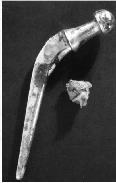
tabl 15. Corrosion of a hip joint from stainless steel ( J. Walczak et al., 1998).
