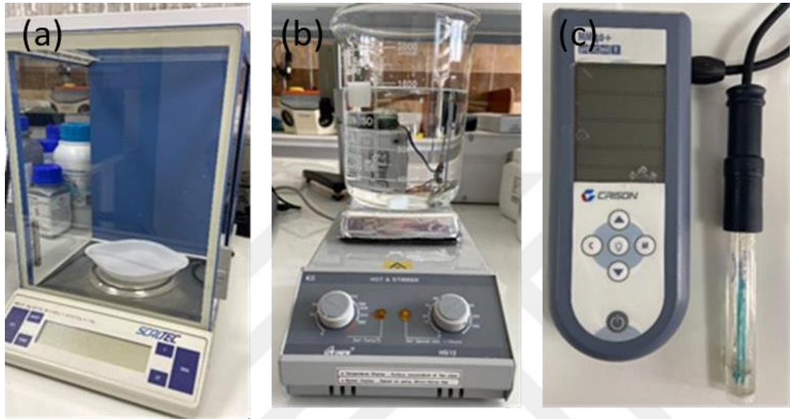
Figure 24. Used devices for preparation of HBSS, (a) precision balance, (b) heating magnetic stirrer and (c) Ph meter.
